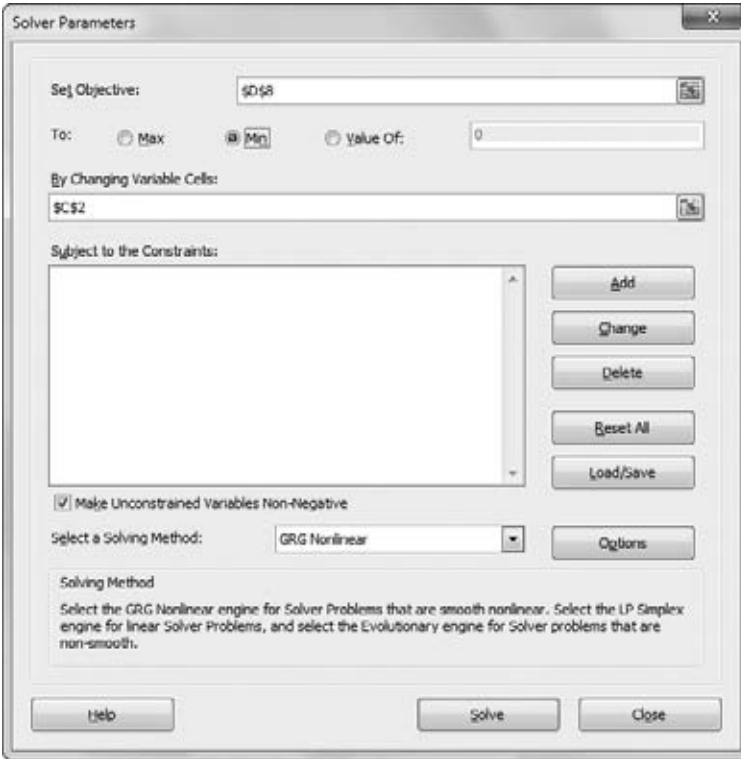
Figure 21-19: Using the Min option tells Solver to make the cell with the total time as small as possible. The only cell that Solver can change is the one that contains the x value. You don't need constraints. Then click Solve; you'll see the result in Figure 21-20.
