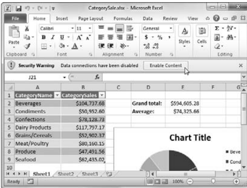
Figure 23-6: This warning message tells you your workbook contains one or more data connections, and that Excel closed them just to be safe. You can switch them back on by clicking the Enable Content button.
