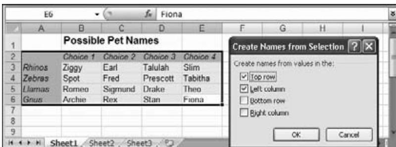
Figure 13-11: You can also use Create Names from Selection with a table of data. In this case, by turning on Left Column , Excel uses each of the animals in column A as the title for a different named range. The Rhinos range, for example, contains cells B3 to E3. If you turn on the "Top row" checkbox, then Excel also creates named ranges for each column, like Choice_1 (cells B3:B6), Choice_2 (cells C3:C6), and so on. It's up to you whether you want to create ranges for row headings, column headings, or both.
