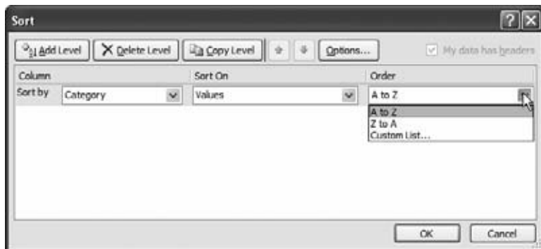
Figure 14-10: To define a sorting key, you need to fill in the column you want to use (in this example, Category). Next, pick the information you want to use from that column, which is almost always the actual cell values (Values). Finally, you need to choose the order for arranging values, which depends on the type of data. For text values, as in this example, you can pick A to Z, Z to A, or Custom List (page 76).
